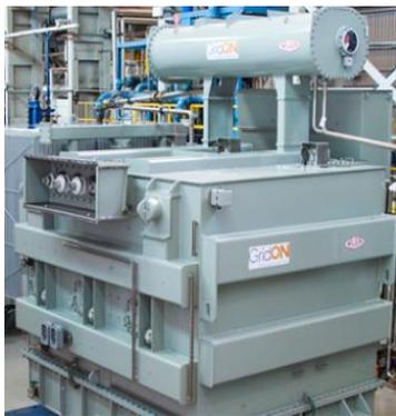
The FCL has undergone a complete factory test, as well as short-circuit testing under rigorous conditions at Ausgrid Testing & Certification lab, a certified high-power test lab. During the tests, the FCL limited 20.2kA first-peak fault current by over 50% and withstood 13.1kA rms (33.4kA peak) prospective fault current for three seconds. Following successful testing, the FCL has been commissioned and energised early April, at WPD's Castle Bromwich primary substation in Birmingham, UK.
